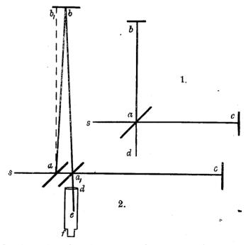
and ca is partly reflected along ad. If then the paths ab and ac are equal, the two rays interfere along ad. Suppose now, the ether being at rest, that the whole apparatus moves in the direction sc, with the velocity of the earth in its orbit, the direction
